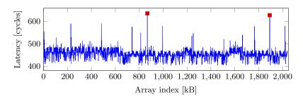
Fig. 2: Access times when alternately accessing two addresses which are 64B apart. The (marked) high access times indicate row conflicts.
