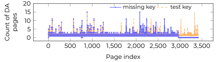
Fig. 4: Traces of the Wasm runtime for the oak key_lookup module with a missing and a test key [72].
